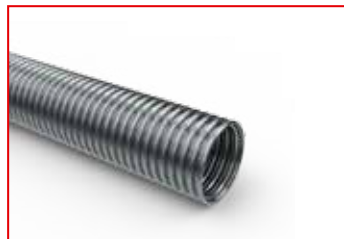
After the tube has been welded, corrugations are formed into the tube to make it flexible
